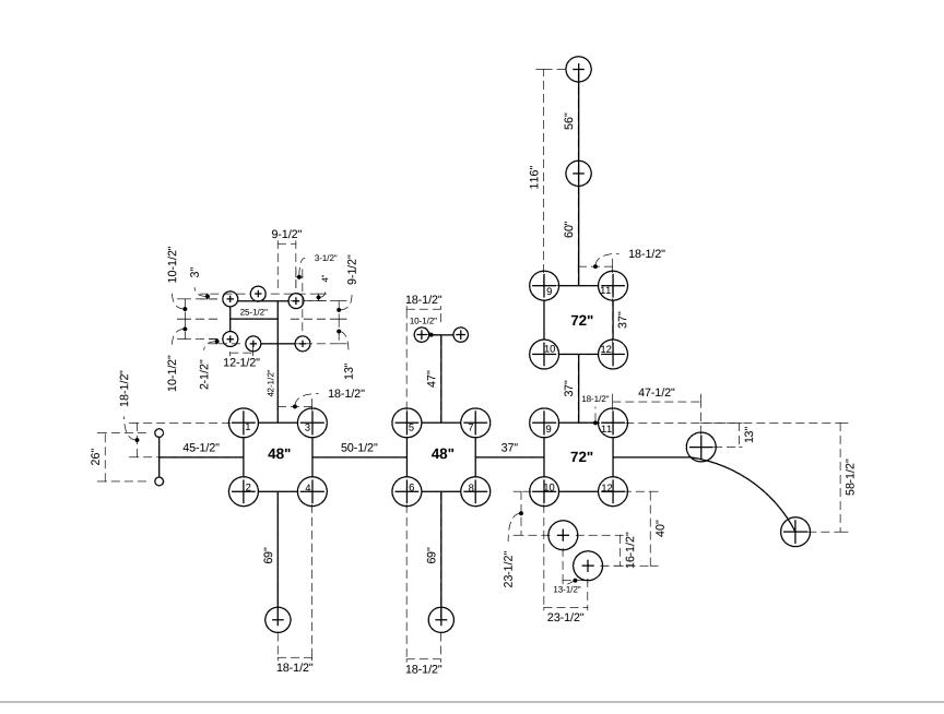
Footer Layout provided as a guide. Measurements rounded to nearest 1/2 inch. For true accuracy, please measure using equipment onsite. Equipment dimensions are subject to change without notice.
