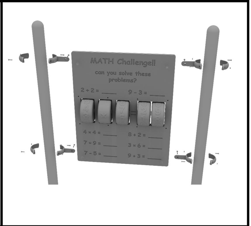
Install four (4) Tube Clamps to the panel following the Clamp Installation Guide.
