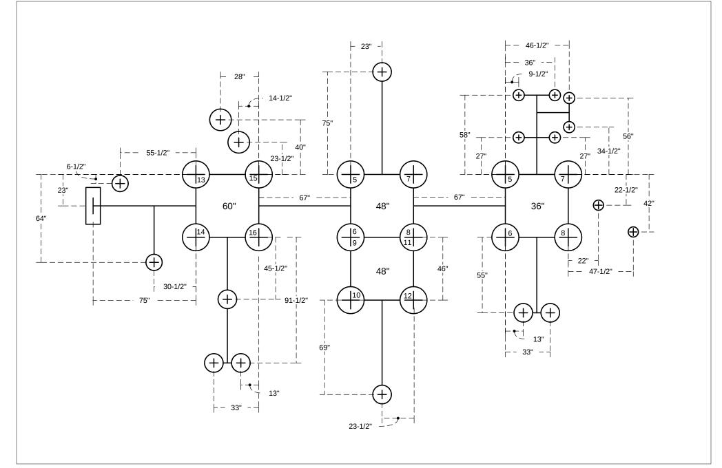
Footer Layout provided as a guide. Measurements rounded to nearest 1/2 inch. For true accuracy, please measure using equipment onsite. Equipment dimensions are subject to change without notice.
