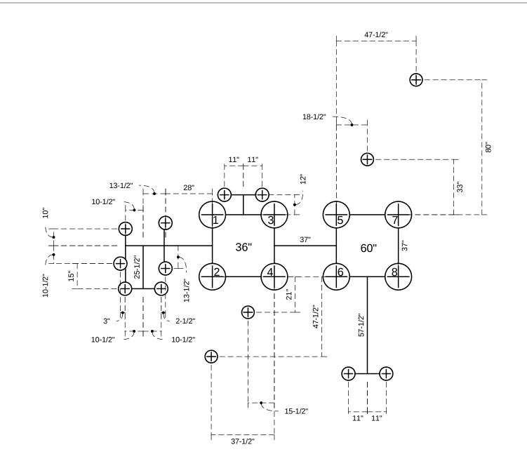
Footer Layout provided as a guide. Measurements rounded to nearest 1/2 inch. For true accuracy, please measure using equipment onsite. Equipment dimensions are subject to change without notice.
