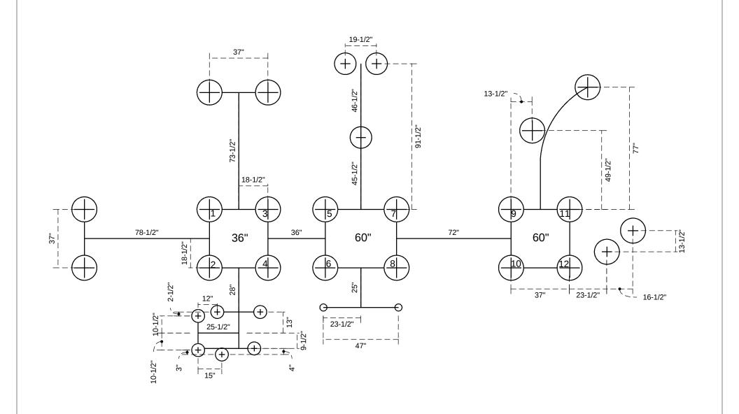
Footer Layout provided as a guide. Measurements rounded to nearest 1/2 inch. For true accuracy, please measure using equipment onsite. Equipment dimensions are subject to change without notice.
