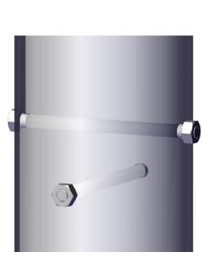
Note: Your post may have two sets of holes. Please install the one threaded rod into one of either sets of holes.
