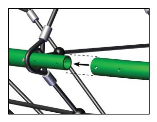
Install four machine screws (N) on each connection of the assembled ring where the two halves join.
