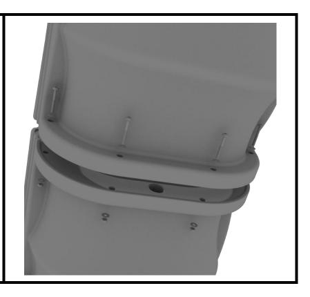
See general installation guide footing information regarding installation of the middle supports, and slide end mount. Insert the middle support into the designated slot under the slide, and tighten the set screws using the provided allen wrench. Repeat this process for the other slide support post.
