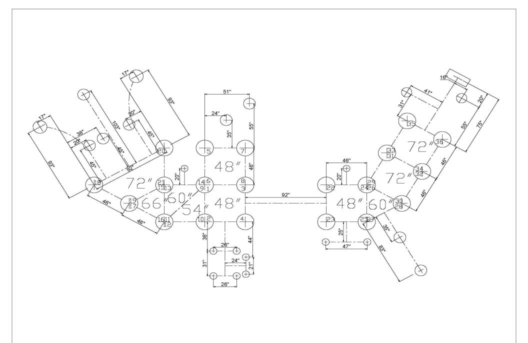
Playground Equipment Footer Layout provided as a guide. Measurements rounded to nearest 1/2 inch. For true accuracy, please measure using equipment onsite. Equipment dimensions are subject to change without notice.
