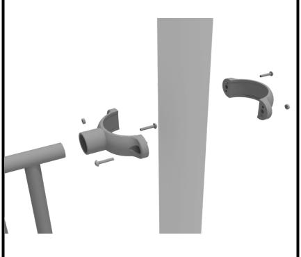
Connect the Net Climber to the designated post using four (4) 3.5inch tube clamps.
