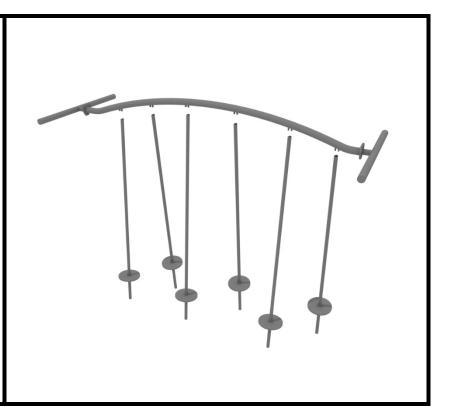
1 Playground Drive Greenfield, IN 46140 1-800-667-0097 Created By: Derick H Date: 10/26/2018 Each of the pebble steps will attach to the top rail using one (1) M10\*55 bolt, two (2) M10 washers, and one (1) M10 lock nut.
