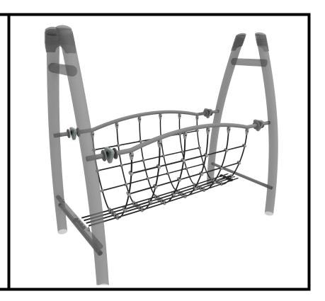
Using the last four (4) longer M10\*75 Bolts and accompanying locknuts, secure the last two Crossbar Supports to the unit.
