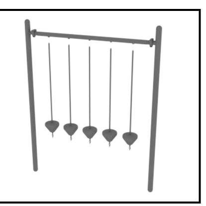
1 Playground Drive Greenfield, IN 46140 1-800-667-0097 Created By: Matt N Date: 3/22/2021 Each of the pebble steps will attach to the top rail using one (1) M10\*55 bolt, two (2) M10 washers, and one (1) M10 lock nut.
