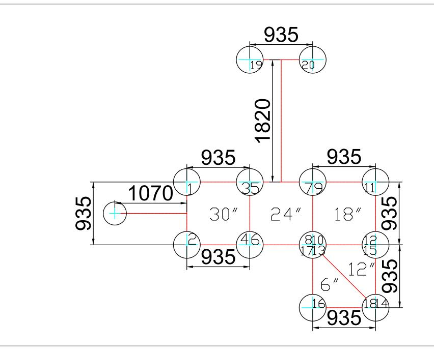
Footer Layout provided as a guide. Measurements rounded to nearest 1/2 inch. For true accuracy, please measure using equipment onsite. Equipment dimensions are subject to change without notice.
