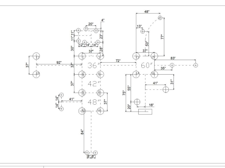
Playground Equipment Footer Layout provided as a guide. Measurements rounded to nearest 1/2 inch. For true accuracy, please measure using equipment onsite. Equipment dimensions are subject to change without notice.
