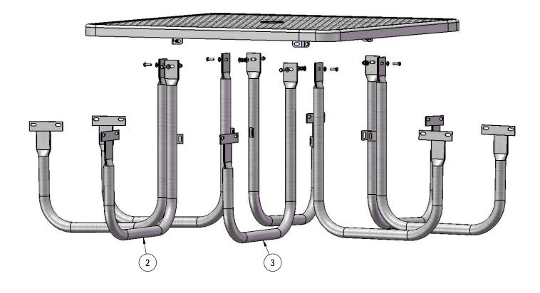
Attach the 358 Legs to the Extension Tabs using specified hardware.
