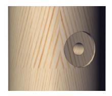
Install a cross tension plate (C) to the inner side holes of each connection (toward Spider Web) using two 3/4 in Torx screws (E) each as shown.
