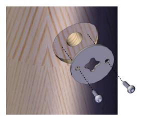
• Find the top connection of one side and pass the chain through its corresponding crossed tension plate, through the post and out the other side. Work the chain through until there are a few links on the outer side.
