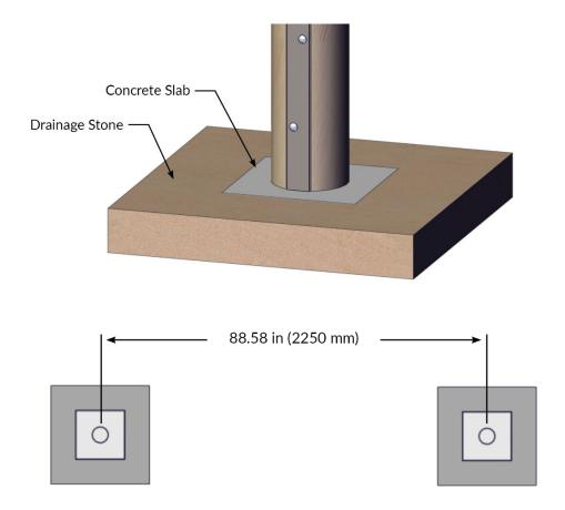
• Using a tape measure, check that the dimension between the center of each connecting post is exactly 88.58 in (2250 mm). Shift the posts on the concrete slabs until the correct measurement is achieved.
