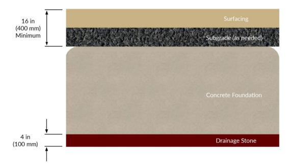
• Place 4 inches (100 mm) of drainage stone evenly on the bottom of each foundation hole.
