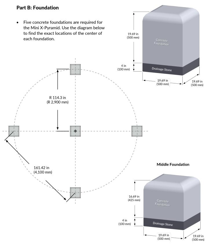
• Dig all five foundation holes to the following dimensions. Depth dimensions include surfacing and 4 inches (100 mm) for drainage stone. The depth indicated for each foundation is measured from the top of the intended surfacing level.
