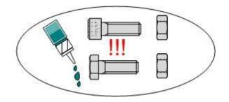
Glue all screws, nuts and sleeves with loctite. No less than 5 drops! (Except for Nyloc nuts)
