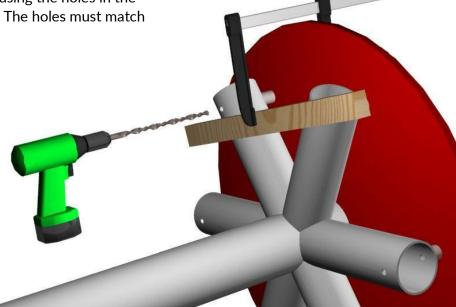
• With all 8 mm holes drilled through the stanchions into the platform, widen the holes in the platform by drilling them with a 17 mm drill bit from the other side. Do not drill through the holes in the stanchion with the 17 mm drill bit.
