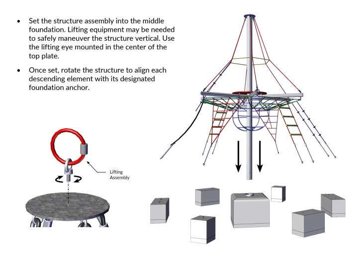
• Check the structure post with a level to ensure that it is sitting straight. Remove the lifting eye from the top plate when finished.
