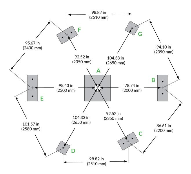
• Dig all seven foundation holes to the following dimensions. Depth dimensions include surfacing and 4 inches (100 mm) for drainage stone.
