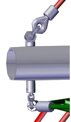
Attach the 6 top eye nuts of the guy rope assembly to the underside of the top plate with 6
