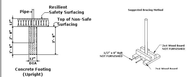
IF RESILIENT SURFACING IS TO BE LESS THAN 12", THEN ADDITIONAL PIPE SHOULD BE PUT IN CONCRETE TO MAINTAIN PROPER FINISH GRADE FOR EQUIPMENT.
