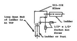
STEP #3: Stand upright & brace in footing holes. Attach braces to legs to hold proper height. Length of pipe below intended level of resilient surfacing
