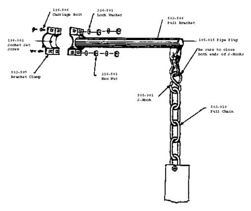
Attach clamps to Top Rail of Swing Frame so that Pull chain hangs in front of wheelchair position users will normally face. Bottom of pull chain has a swivel snap for attaching the end to a chain of the wheelchair swing platform to hold it out of the way for entering and exiting the platform.
