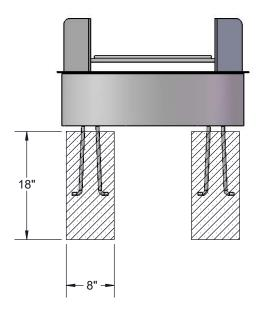
Attach the ground staples to the Fire Ring before inserting then into the concrete footings.
