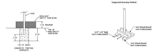
• If resilient surfacing is to be less than 12", then additional pipe should be put in concrete to maintain proper finish grade for equipment.
