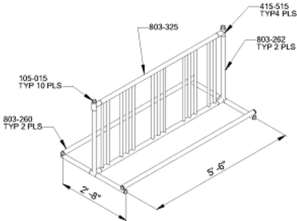
Main Frame, legs and spacers are 1 5/8" O.D. hot galvanized welded pipe with 3/4" O.D. hot galvanized ladder rungs. Spacing between tire posts is 3" center-to-center for small gap, 8 1/2" center-to-center for large gap.
