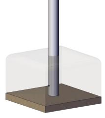
With measurements checked, and all posts in place, straight and level, pour the concrete foundations.
