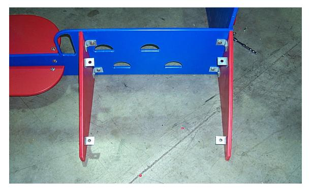
14. Now attach the ladder (M) to the 4 corner brackets and tighten all hardware.
