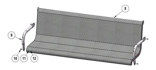
While waiting for Footings to cure attach the 967 Armrest to the 967 Bench using the specified hardware.
