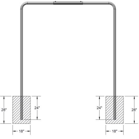
After Step 1 place 967 Legs into footings and pour the estimated amount of Concrete to fill footings. While curing continue to Step 2.
