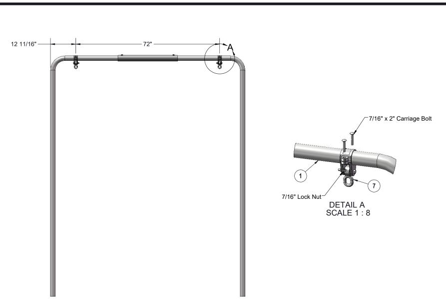
After Footings have cured attach the 2- Swing Hangers to the 967 Legs using the specified hardware. At the appropriate distance apart from each other.
