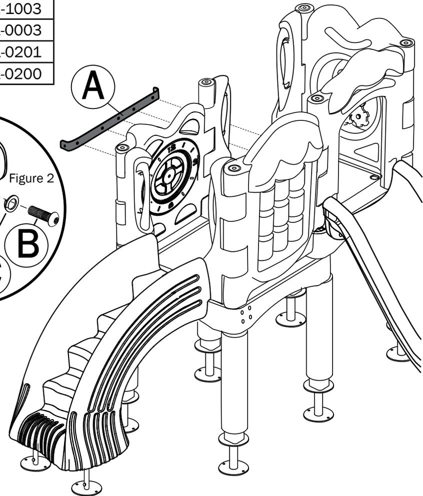
1. Align holes in Vine Climber Bracket(A) with inserts in Deck
