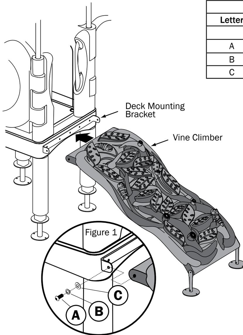
1. Insert Bolt(A), Lock Washer(B) and Flat Washer(C) into hole in Deck Mounting Bracket and into threaded insert in Vine Climber.
