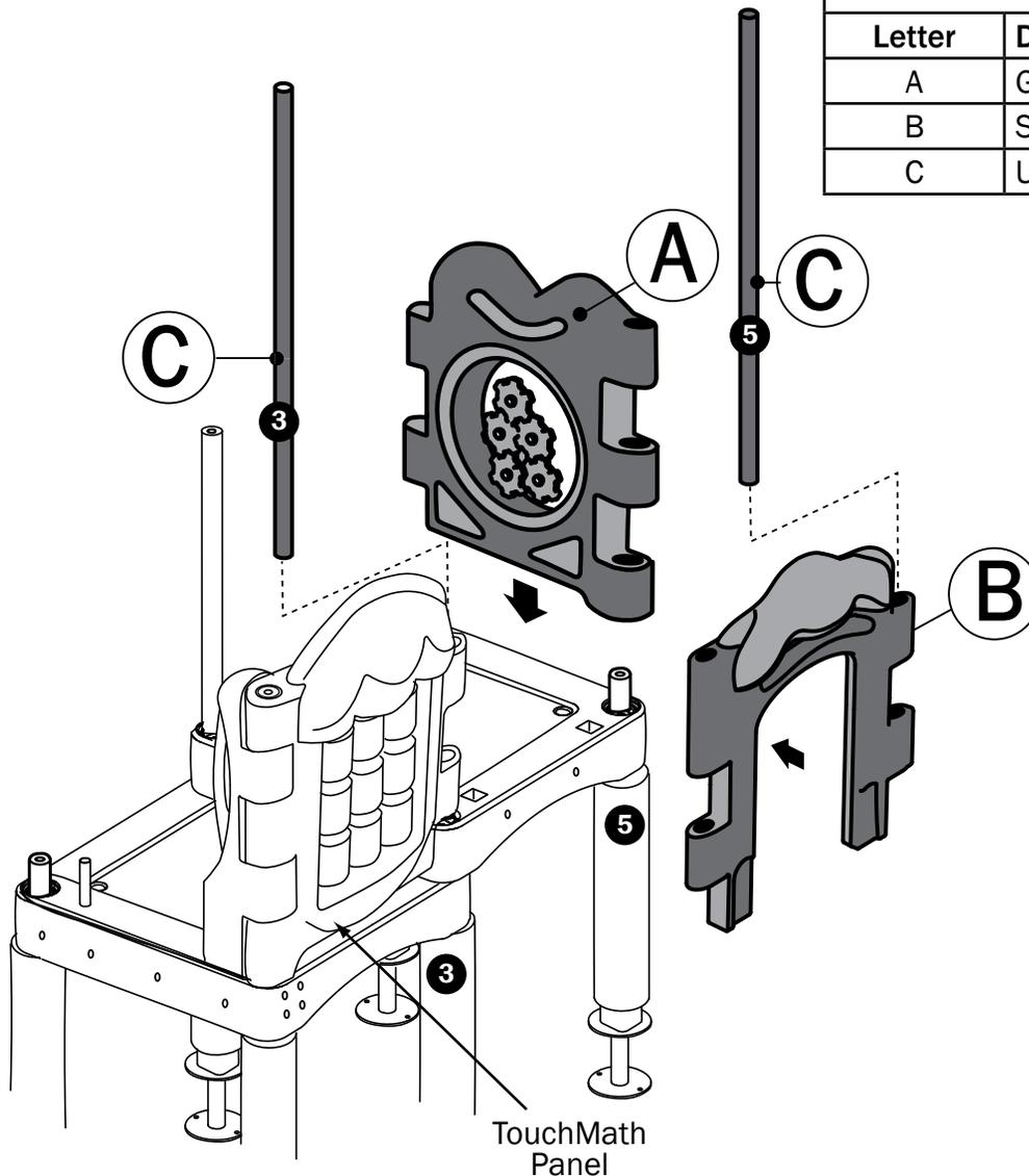
1. Lower Gear Panel(A) onto Lower Post #5.
