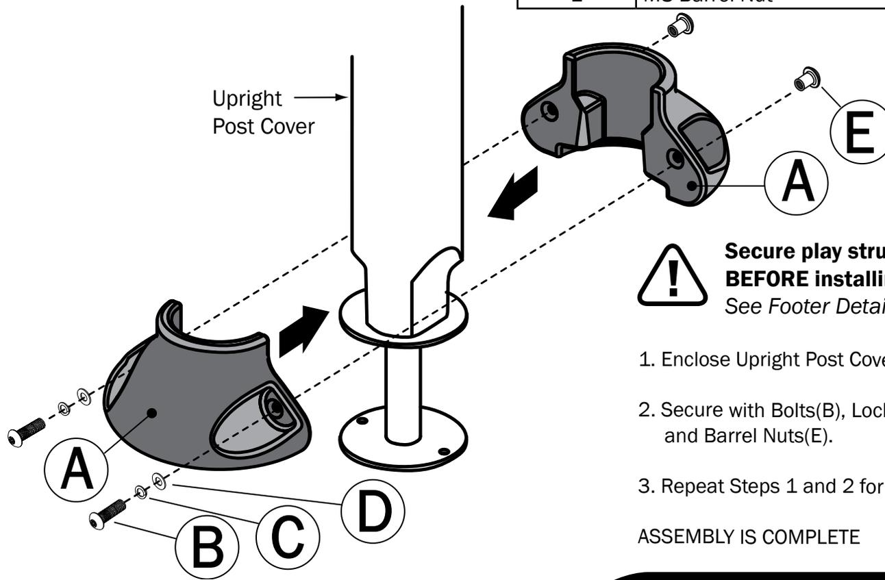
**Secure play structure to the ground BEFORE installing Footer Covers(A).**
