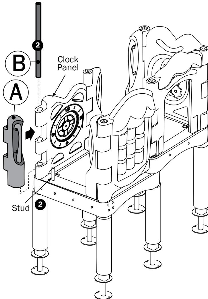
1. Align hole in underside of Climber Handhold(A) with stud on Climber Mounting Bracket .
