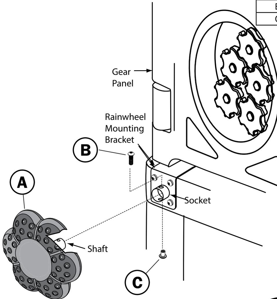
1. Insert shaft of Rainwheel(A) into socket of Rainwheel Mounting Bracket.
