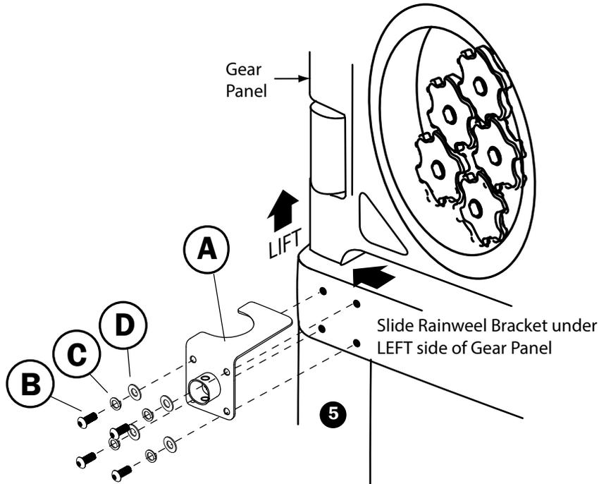
1. Lift LEFT side of Gear Panel on Post #5.
