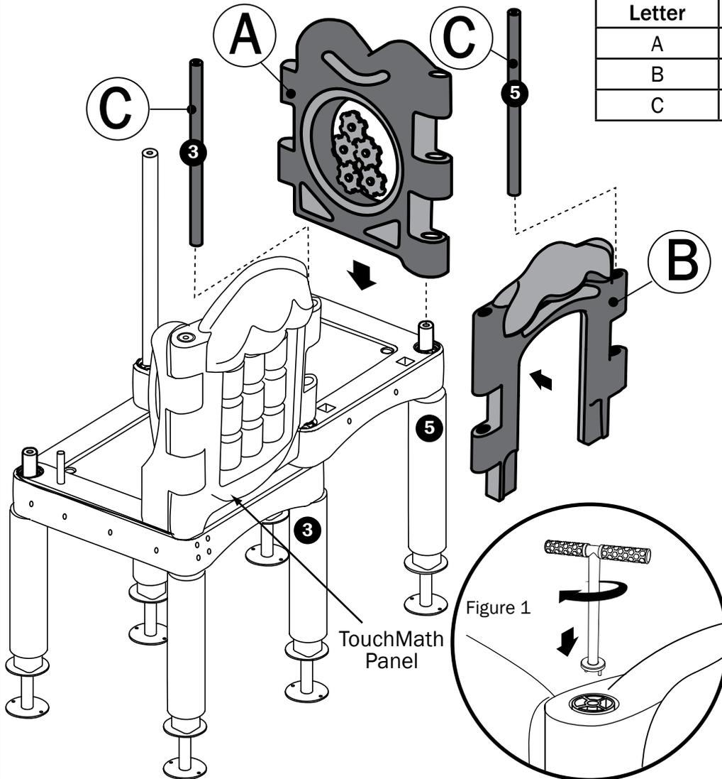
1. Lower Gear Panel(A) onto Lower Post #5.
