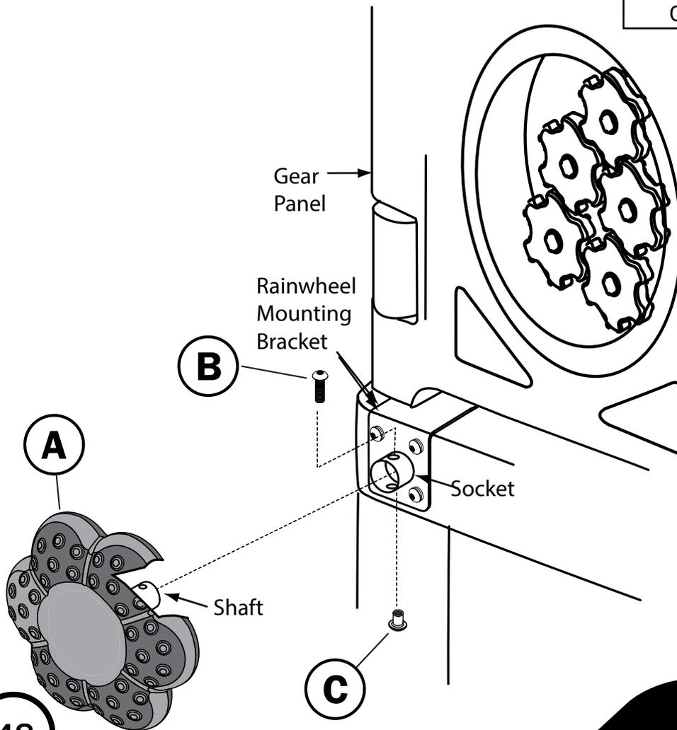
1. Insert shaft of Rainwheel(A) into socket of Rainwheel Mounting Bracket.
