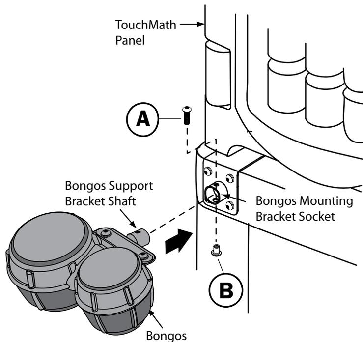
1. Apply Loctite adhesive to threads of Bolts(A).
