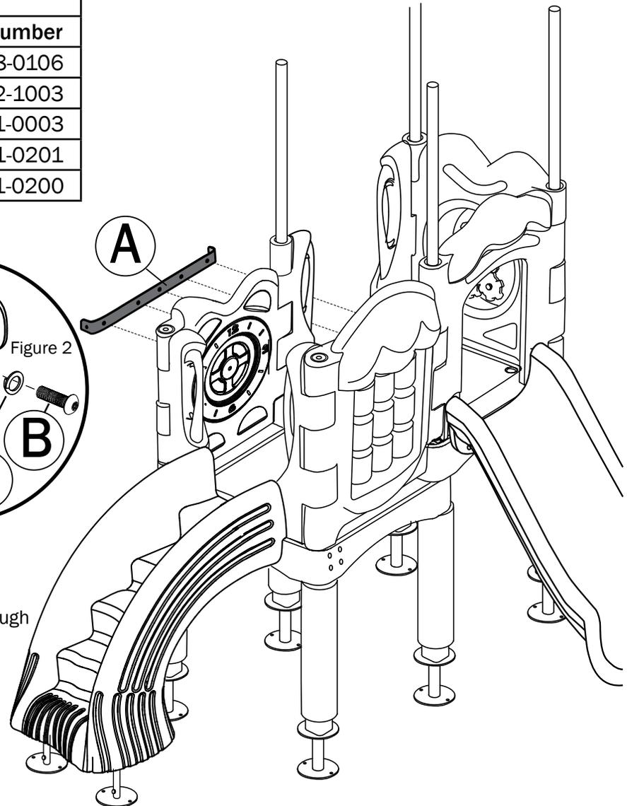
1. Align holes in Vine Climber Bracket(A) with inserts in Deck.
