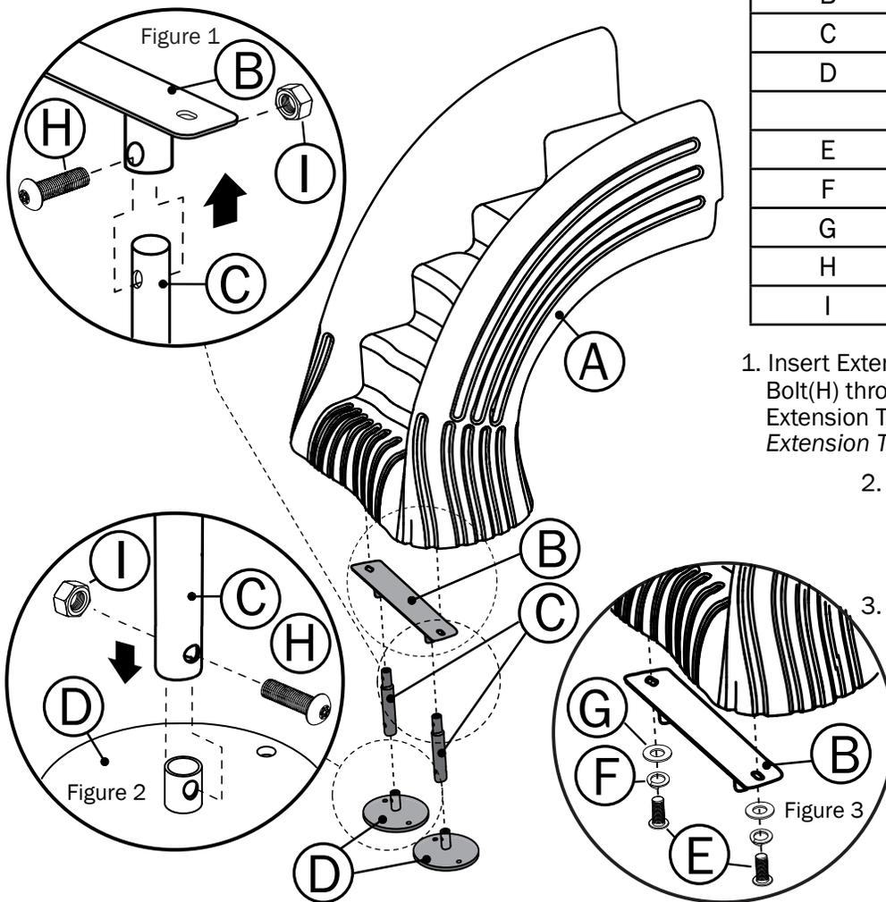
1. Insert Extension Tube(C) into Stump Climber Mounting Bracket(B). Insert Bolt(H) through larger hole in Stump Climber Mounting Bracket(B), through Extension Tubes(C) and secure with Lock Nut(I). Repeat for other Extension Tube(C). See Figure 1.
