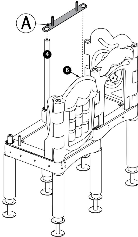
1. Lower Climber Handhold Bracket(A) onto Lower Posts #4 and #6.
