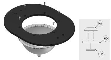
2. Attach Metric Table (A) to the top of the Bowl Tables (D & E) using (6) 5/16-18 X 1-3/4 SS w/Patch(HC), (6) 3/4" Flat Washers(HD) and (6) 5/16"-18 Nylon Lock Nut SS(HB).
