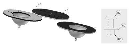
**3.** Attach Table Legs (B) to the bottom of each table using (2) 5/16-18 X 1 SS w/Patch (HA), (2) 1" Flat Washers(HD) and (2) 5/16"-18 Nylon Lock Nut SS(HB) per table leg.
