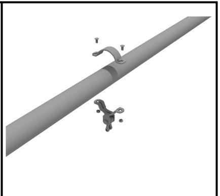
Loosen hardware on swing hanger pendulum and attach chain.
