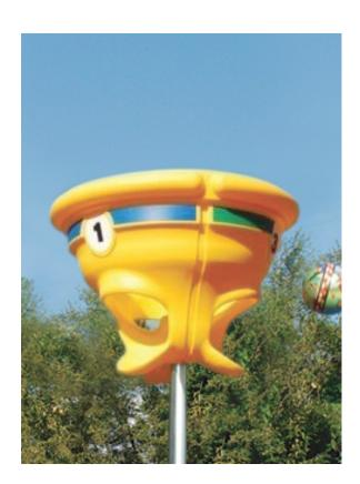
The Funball shall feature a 30" OD rotomolded polyethylene shell with UV stabilizer molded in for color retention. The 3 ball openings hall is 10.5" OD. Post shall be 3.5" OD galvanized steel.
