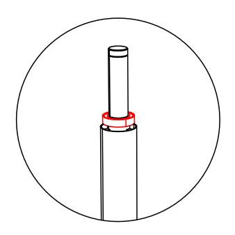
Place the primary bearing assembly over the end of the support post.
