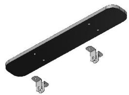
2) Slide the shelf onto the base sandwiching the base between the L-brackets. Attach the shelf using (2) 5/16-18 x 1 Torx Head Bolt (HE) and (2) 5/16-18 T-Nut SS (HF). (As Shown)
