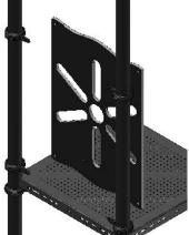
3) Level and adjust all clamps as needed and then tighten around poles and tighten to panel.
