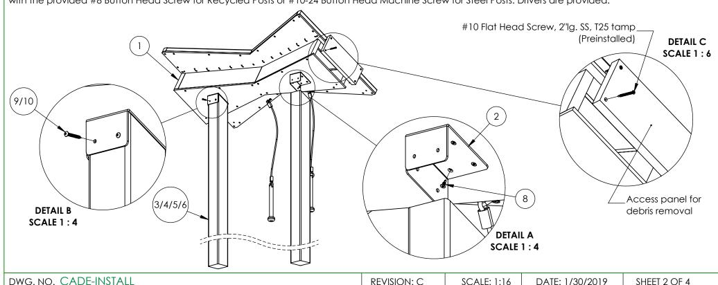
**Step 1:** Excavate two 10" diameter holes, 36" deep, and 30" on center at the installation location. Contractor can modify Post to desired height.
