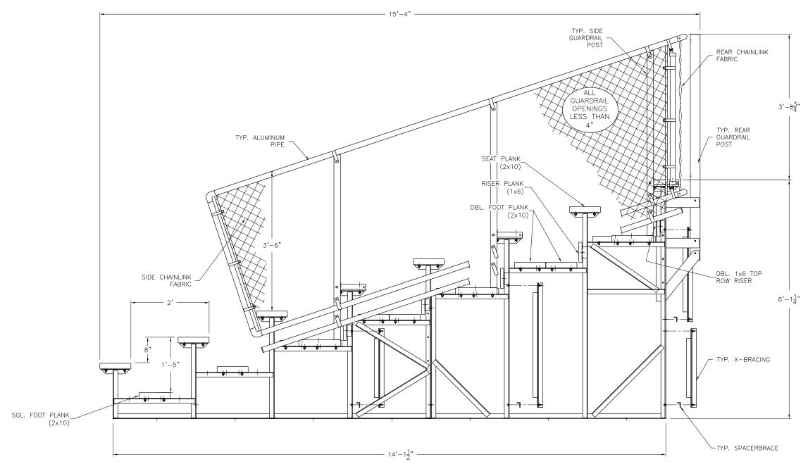
**NOTE:** ILLUSTRATION SHOWN WITH SINGLE FOOT PLANK ROWS 2 & 3, DOUBLE FOOT PLANK ROWS 4-8, 1x6 RISER (ROWS 4-7), DBL. 1x6 RISER (ROW 8), & CHAINLINK GUARDRAIL. PLEASE REFER TO ATTACHED SPECIFICATIONS FOR FEATURES INCLUDED WITH YOUR SPECIFIC BLEACHER.
