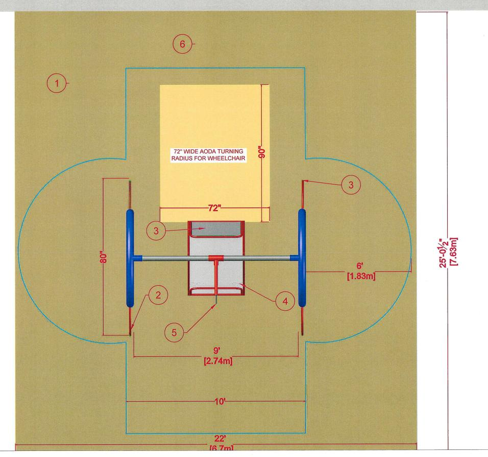
ENGINEERED WOOD FIBER PROTECTIVE SURFACING 2 CONTRASTING PROTECTIVE RAILS 3 28" RAMP, DOUBLING AS SEAT BACK 4 WHEELCHAIR SECURING Q-STARPS 5 ANCHORED PROPULSION ROPE 6 SWING BAY MATT - 72" x 90"
