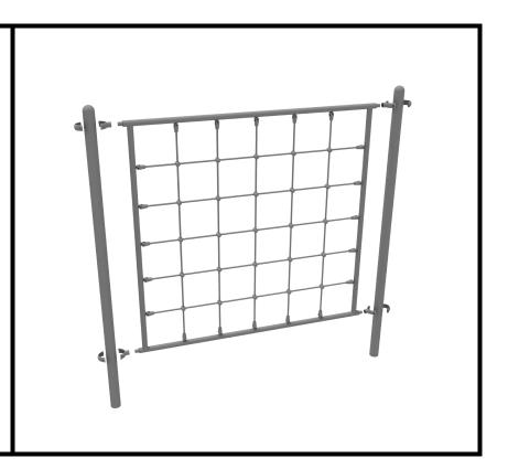
See general installation guide regarding footing information for the cyclone challenger climber. Then, attach each support mount to the bottom of the climber using one (1) M10\*20 bolt, one (1) M10 spring washer, and one (1) M10 washer per mount.
