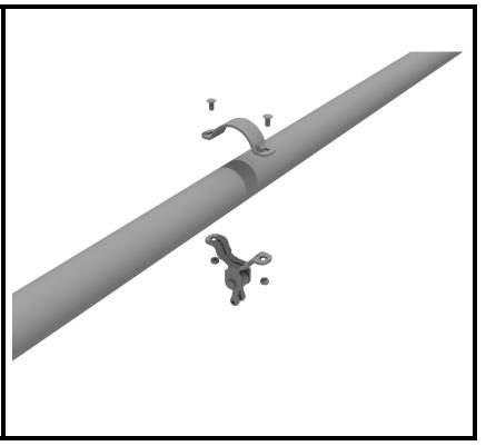
Loosen hardware on swing hanger pendulum and attach chains.
