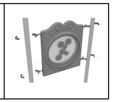
Connect half of the tube clamp to the component using one (1) M8\*30 bolt. Then, using the other half of the flat clamp and the hardware provided in the clamp hardware bag, attach the backside of the flat clamp around the post.
