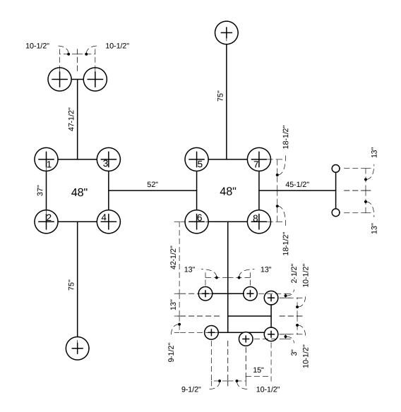
Footer Layout provided as a guide. Measurements rounded to nearest 1/2 inch. For true accuracy, please measure using equipment onsite. Equipment dimensions are subject to change without notice.
