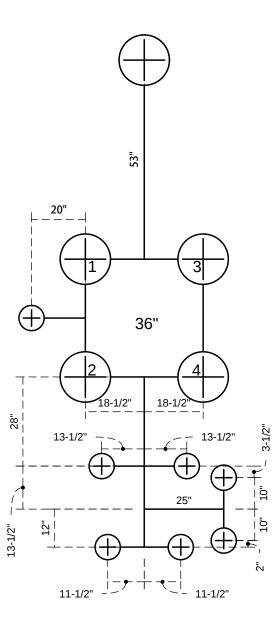
Footer Layout provided as a guide. Measurements rounded to nearest 1/2 inch. For true accuracy, please measure using equipment onsite. Equipment dimensions are subject to change without notice.
