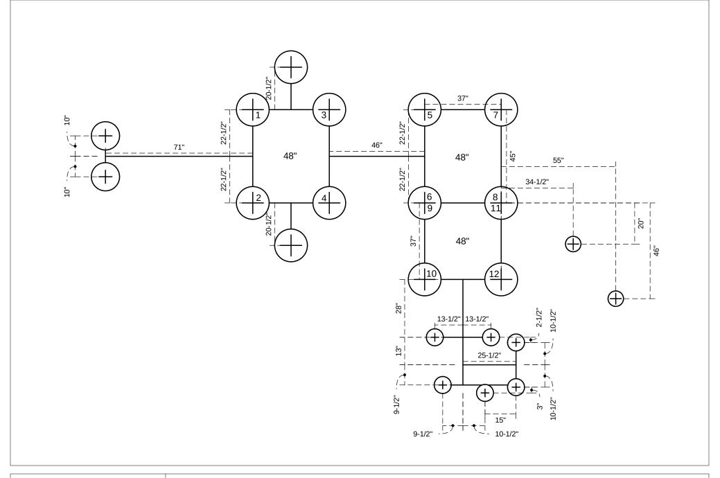
Footer Layout provided as a guide. Measurements rounded to nearest 1/2 inch. For true accuracy, please measure using equipment onsite. Equipment dimensions are subject to change without notice.
