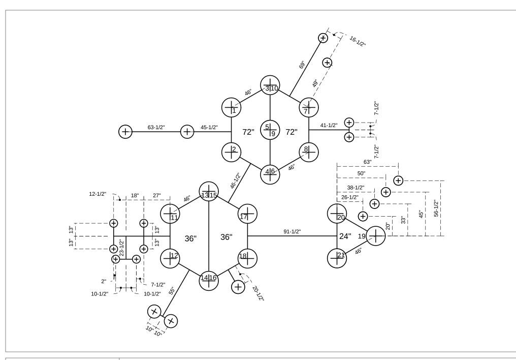
Footer Layout provided as a guide. Measurements rounded to nearest 1/2 inch. For true accuracy, please measure using equipment onsite. Equipment dimensions are subject to change without notice.
