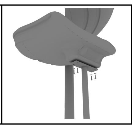
See general installation guide regarding footing information for slides and support posts. Connect the Spiral Slide to the Spiral Slide Deck using three (3) M10\*20 Bolts, three (3) M10 Spring Gaskets, and three (3) M10 Washers.
