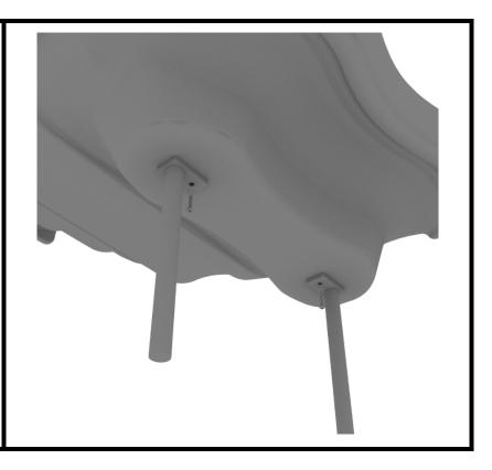
Then, attach the slide to the deck extension using four (4) M10\*45 bolts, eight (8) M10 washers, and four (4) M10 lock nuts.
