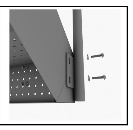
Attach the deck climber extension to the proper deck using four (4) M10\*25 bolts, eight (8) M10 washers, and four (4) M10 lock nuts.
