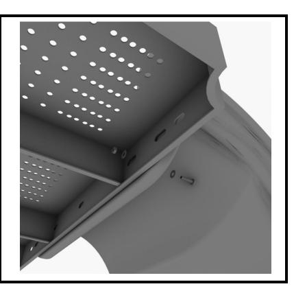
Using one (1) M8\*45 bolt, one (1) M8 washer, one (1) M12 washer, and one (1) M12 Inner hex spiral nut, attach the slide to one side of the slide hood. Repeat this process for the other side of the slide. Make sure all bolts are properly tightened.
