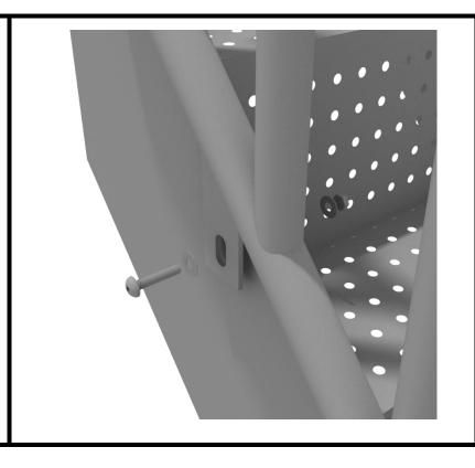
Using two (2) M10\*25 bolts, four (4) M10 washers, and two (2) M10 lock nuts, connect the bottom of the handrail to the stair.
