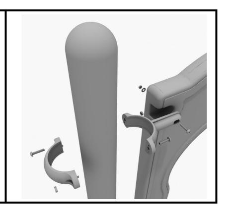
Using the hardware pre-attached to the slide, connect the two sections of the slide together.
