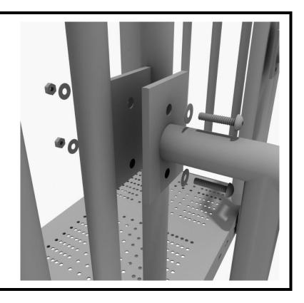
Using one (1) M10\*25 bolt, two (2) M10 washers, and one (1) M10 lock nut, attach the top of the stairway to the deck on the opposite side of the posts. Repeat this step for remaining attachment points.
