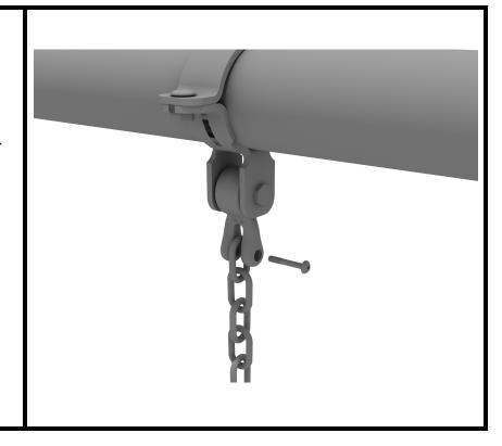
Loosen single clevis hardware and attach belt seat. Re-tighten single clevis hardware. Repeat for bucket seat.
