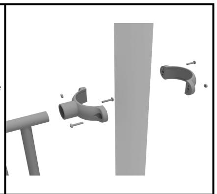
Connect the Spider Web Climber to the designated post using four (4) 3.5-inch tube clamps.
