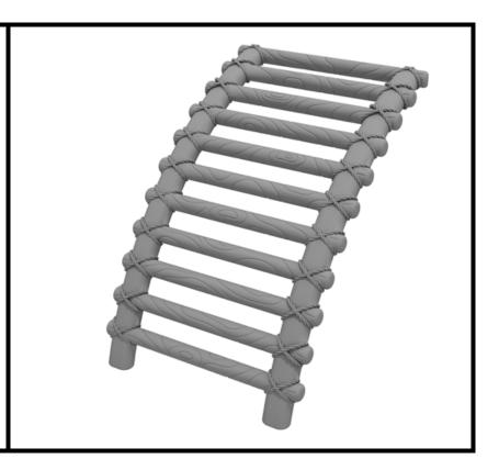
Using two (2) M10\*20 bolts, two (2) M10 spring gaskets, and two (2) M10 washers, attach the bottom of the bamboo climber to the climber end mounts.
